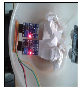
A smart waste bin with HC-SR04 and gas sensors.
